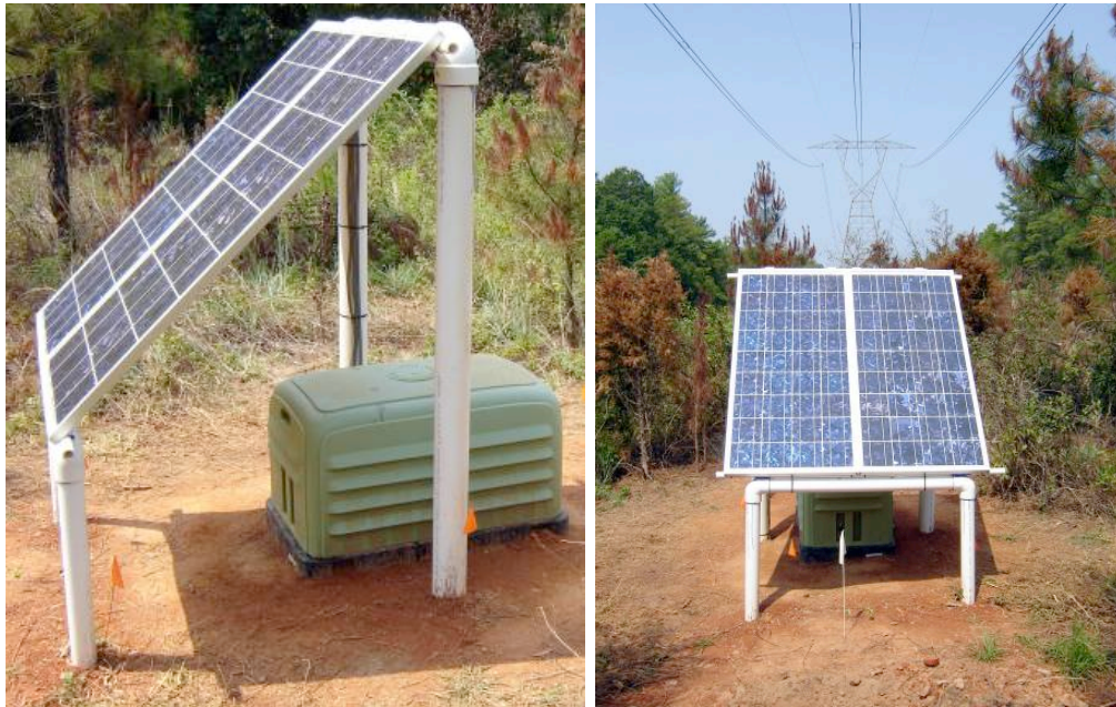
Figure 5. Solar panel and prototype electronics package containing ADCs, a computer and a wireless data link. This will be replaced by a second-generation electronics package which will be installed underground, and will have much lower power consumption allowing the use of a smaller solar panel.
