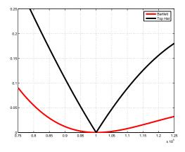
Fig. 3. Expanded view of top hat window versus Bartlett at the nulls.
