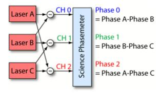
Fig. 5. Block diagram of phasemeter linearity test
