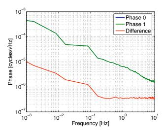
Fig. 8. Measurement of the same input on two different channels, and the difference between the two inputs. The noise on Phase 0 and Phase 1 is due the signal generator; the noise of the difference is due to the ADC jitter.
