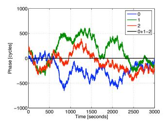
Fig. 6. Sample time series showing the phasemeter measurement from three correlated lasers, and the result of adding the three phase outputs correctly.
