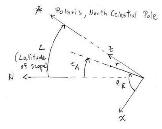
(I corrected a mistake in this diagram and in the following step. The angles didn't add up right.) For the conversion  $e_A \rightarrow e_E$  first note that the angle from the x axis to the z axis is 90 degrees so
