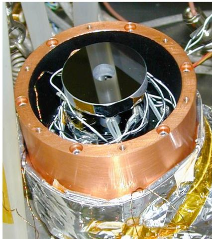
Fig. 3. View of the donut-shaped mirror supported by three piezo-electric actuators, ready for cryo-testing. The actuators and mirror are instrumented with temperature sensors. The copper container has a cover (with holes to allow laser beams to enter) so that the entire sample assembly is in a homogeneous cryogenic environment.
