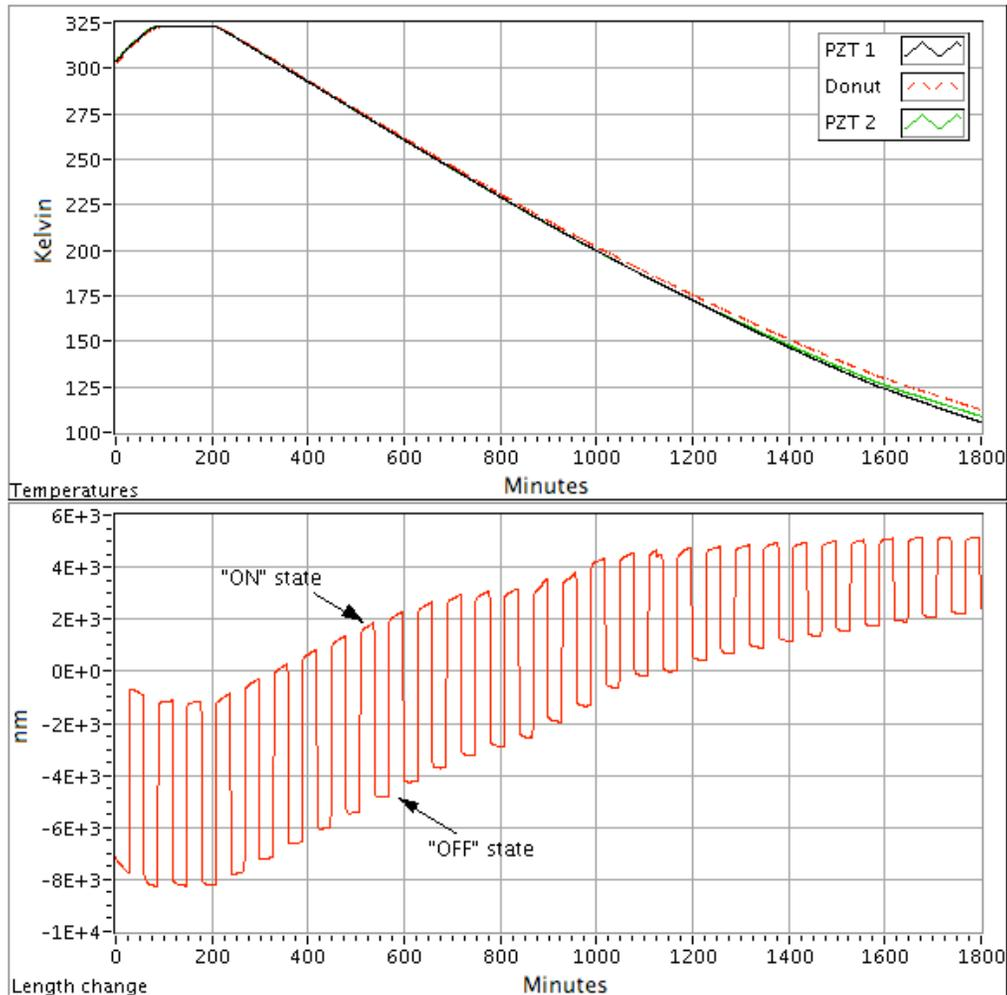
Figure 4. Raw data from PZT actuator test. Upper plot shows sample and “donut” mirror temperatures. Lower plot shows relative displacement of donut caused by actuator extension and CTE. The square-wave like displacement is due to the square-wave voltage applied to the actuators. The increasing trend in the displacement is due to the decreasing temperature causing the actuators to lengthen, indicating that these actuators have a negative CTE.
