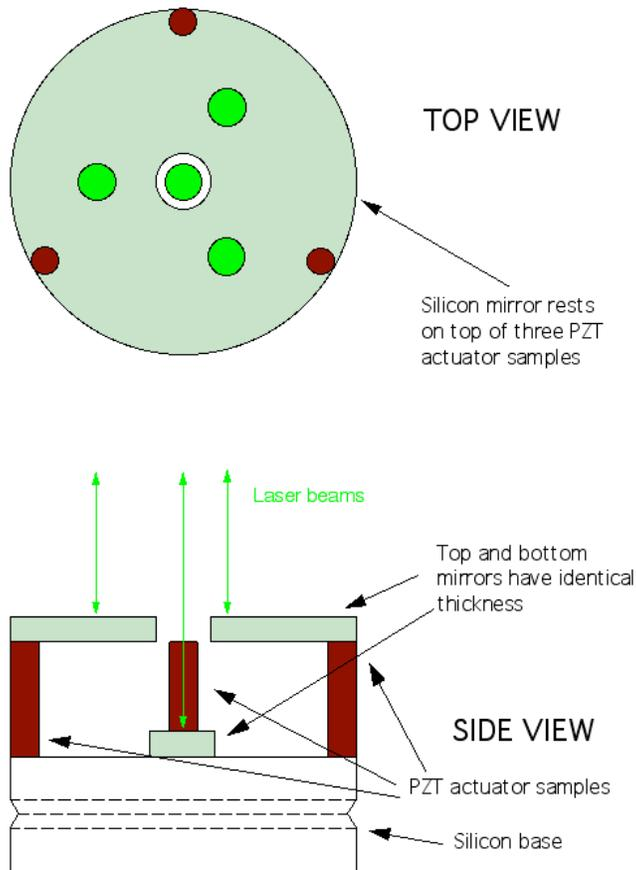
Fig 2. Modified configuration used for actuator testing. Three identical actuators support a mirror with a central hole (the “donut”). This mode requires that the three actuators maintain lengths equal to a few microns, a requirement that is easily achieved by adding small offsets to the voltages on the actuators. The central laser beam reflects either from the base or, as shown here, from a small mirror of thickness and composition identical to the donut, to compensate for the donut’s CTE.
