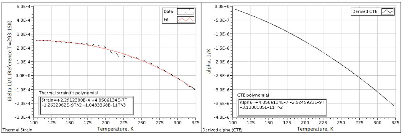
Fig 7. On state strain (referred to 293.15 K) and CTE.
