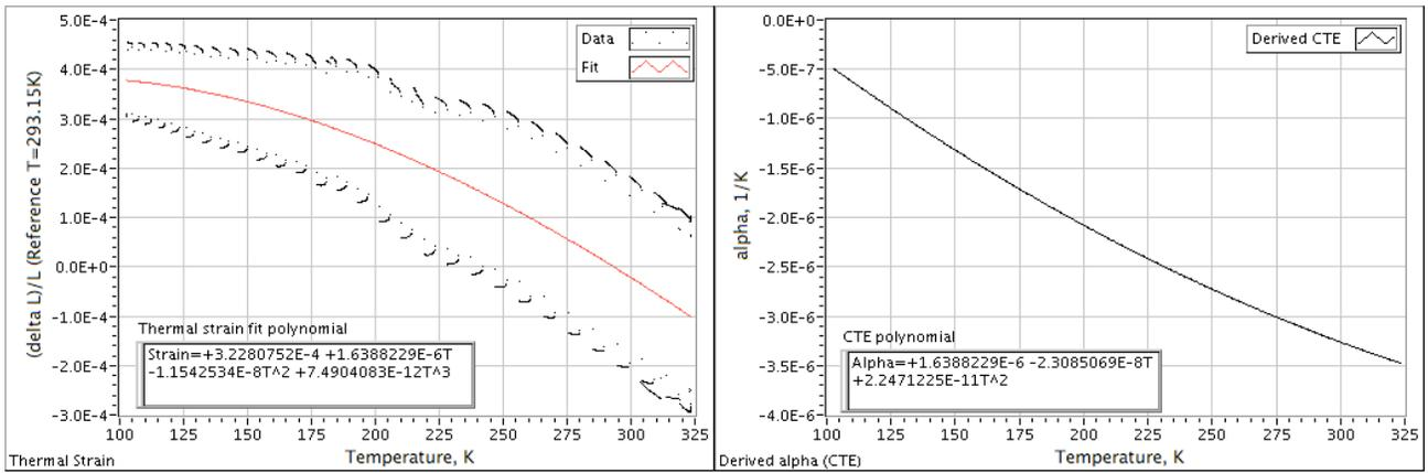
Fig 5. On and off-states “averaged” strain (referred to 293.15 K) and CTE. The fitter that produced the polynomial (red curve) used both the on-state data (upper clusters of data points) and the off-state data (lower clusters). Hence the fit is a compromise between the two states, very nearly the average.
