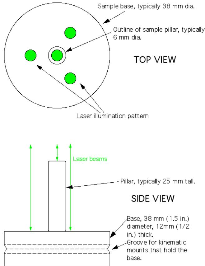
Fig 1. Normal configuration of samples for thermal strain and CTE measurement. Because this setup requires that the top of the sample be polished to mirror finish, it does not work well for actuators.
