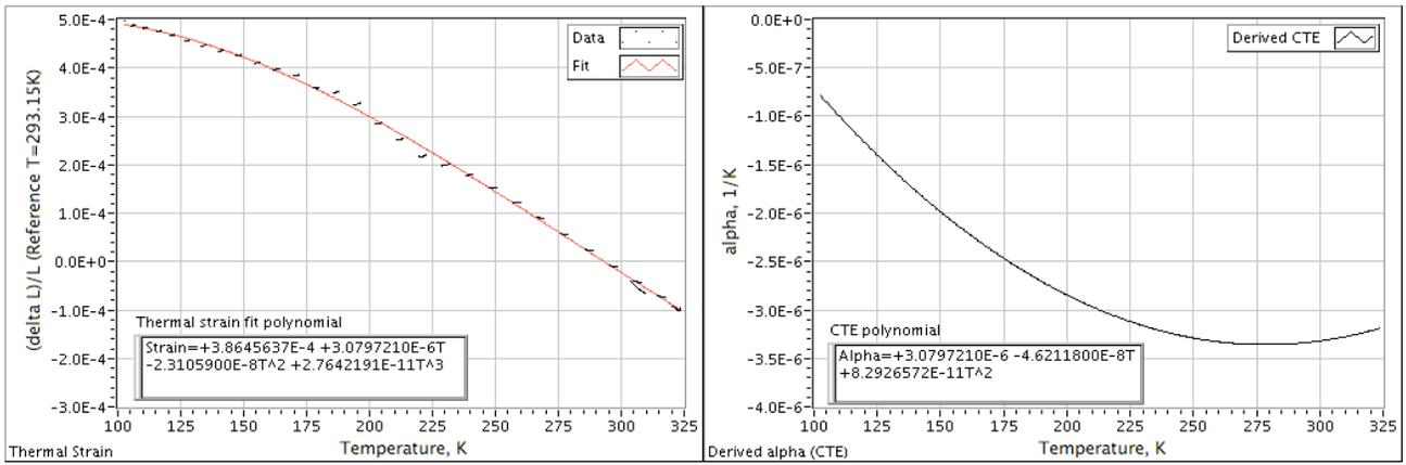
Fig 6. Off state strain (referred to 293.15 K) and CTE.
