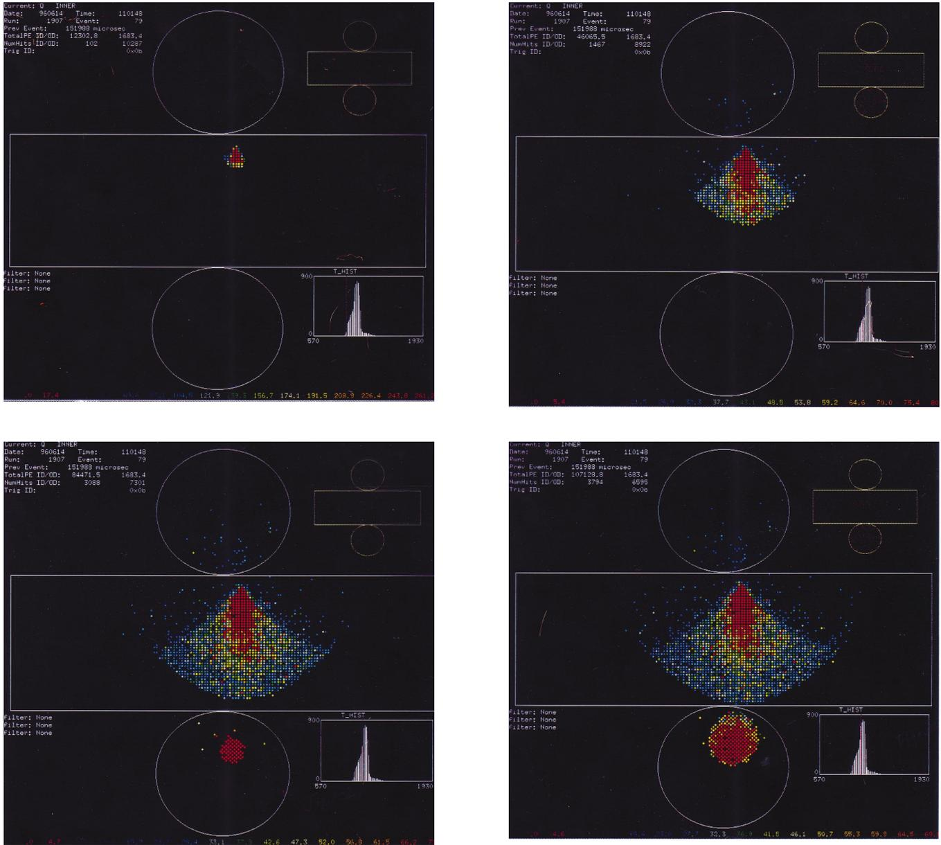
FIG. 4. (Color) Progress of a muon through the Super-KamiokaNDE detector: (4-1) Muon that has just entered Super-KamiokaNDE; (4-2) same muon 50 nanoseconds later; (4-3) muon has reached the bottom.
