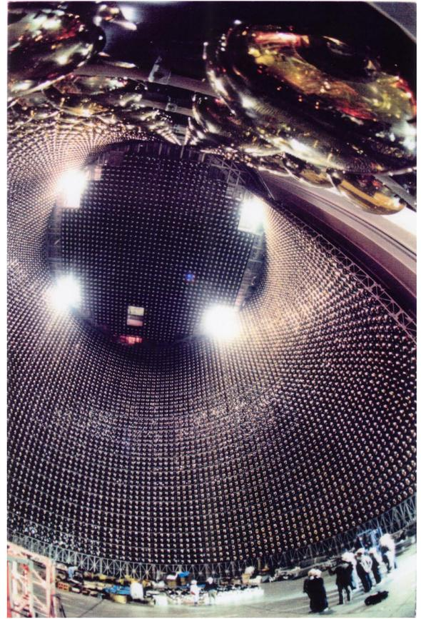
FIG. 3. (Color in online edition) The interior of Super-KamiokaNDE through a fish-eye lens.
