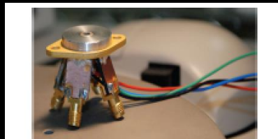
FIG. 3. Photograph of a prototype quadrant photoreceiver manufactured by Discovery Semiconductors.
